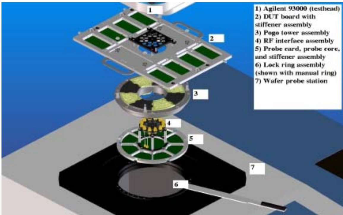
Figure 5. An overview of the wafer probe card hardware assembly setup. (courtesy of Agilent Technologies)
